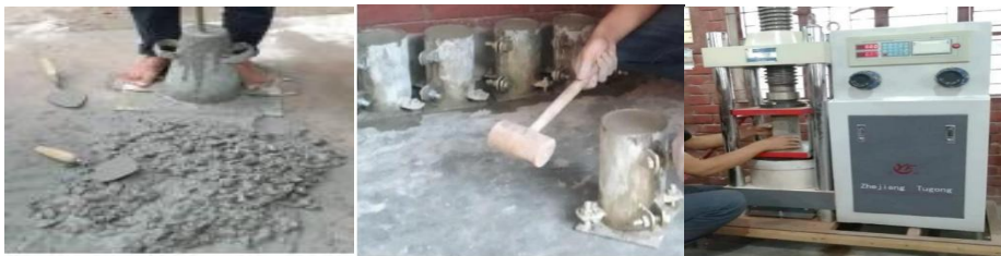
Figure 3: Sample preparation and test set up for compressive strength test
