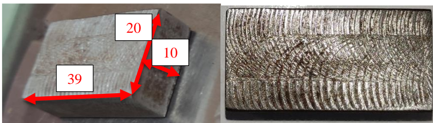
Fig. 1: Sample of Mild Steel Plate taken for the experiment (dimension and roughness)
